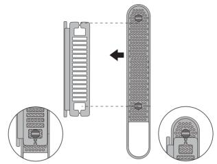
The bottom Mounting Knob thread in the hole and the top Mounting Knob sits on the groove.
